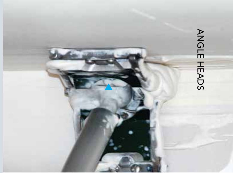
"Fool Proof" Locking Mechanism locks Angle Head on the ball
